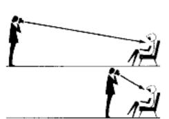
**Substitute reading:** If a close-up reading is not possible, point the camera at a substitute object of average contrast and under the same lighting. Use the setting obtained for the exposure.
