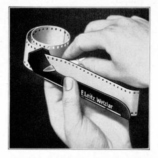
Fig. 26. Trimming Template (Trimming the film for the receiving spool)
